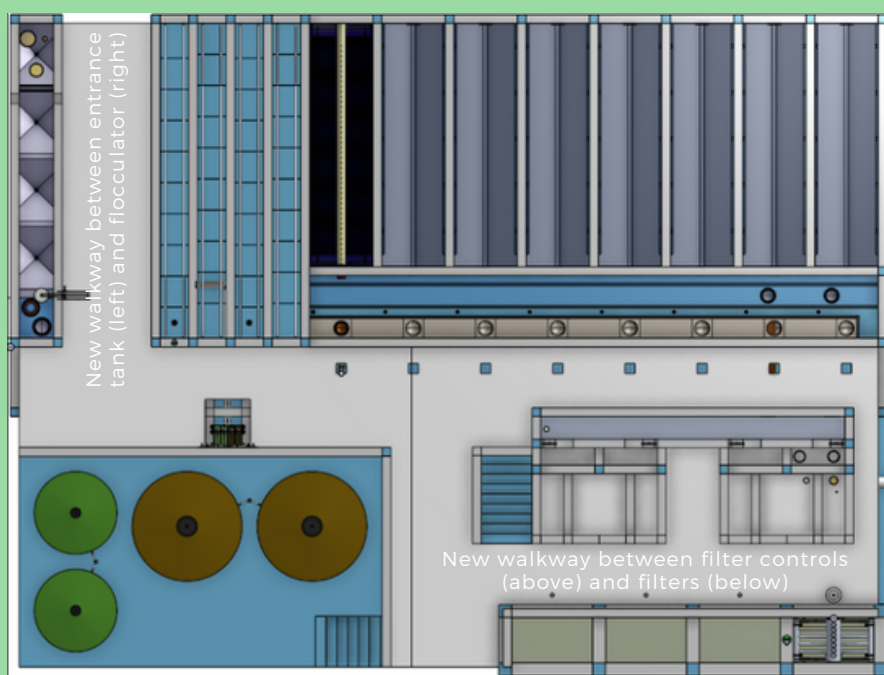
Plan view of the new plant layout. The entrance tank and flocculator are separated by a walkway and the filter controls are moved away from the filter for easier access.
