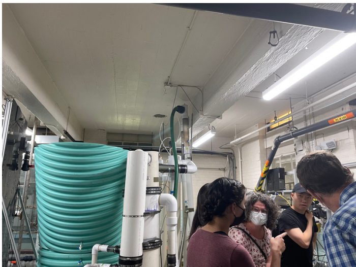
(Left) Pilot plant clarifier made of corrugated pipe (left) and stacked rapid sand filter (right).
